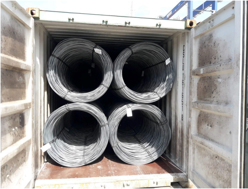
Coils specially formed for container shipment.
