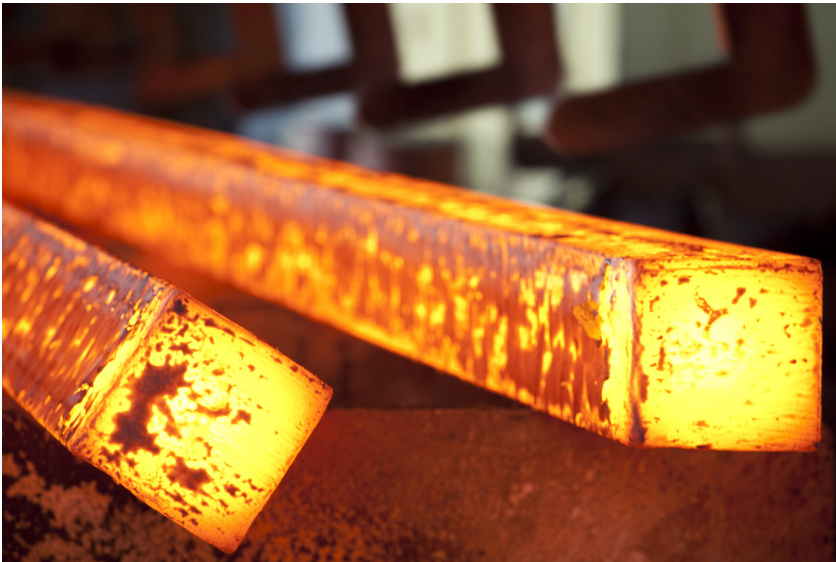
Billets cast on a SMS Concast continuous caster.
