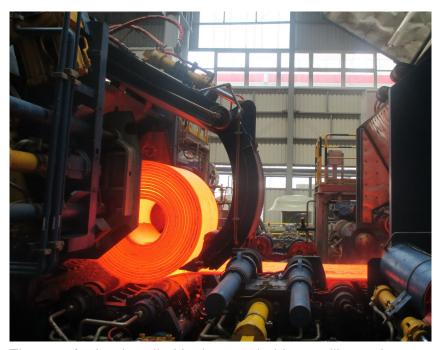
The transfer bar is coiled in the mandrel-less coilbox, where the temperature losses of the inner windings are extremely low.
