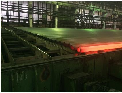
Seamless steel pipes on the cooling bed in the Tagmet PQF® mill.
