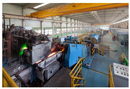
A comparable CONTIROD®\* casting and rolling plant for copper wire.
