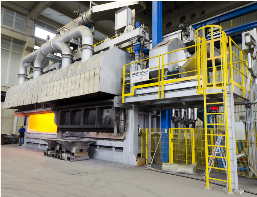
Hertwich multi-chamber melting furnace Ecomelt PS.
