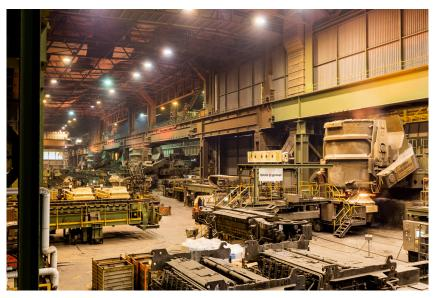
The four continuous casters at the Salzgitter Flachstahl plant were supplied by SMS group. Photo: Salzgitter Flachstahl.
